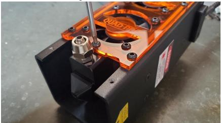
4. Pull off the air assist nozzle. (picture might be different depending on the version of air assist.
