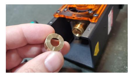
7. Reinstall everything in by putting the lens cover back on, the air assist back on, and the shieling piece back on. To get the air assist nozzle back on, you might need to loosen the two screws on the bottom of the larger shielding piece.
