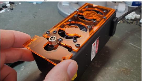
3. Unscrew the screw holding the air assist on.
