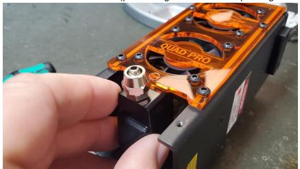
5. This will expose the lens cover. You can clean it or inspect it without removing it or you can remove it. Clean it with a q tip and isopropyl alcohol or micro fiber cloth.
