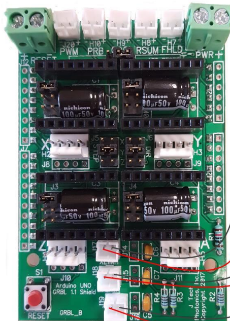
Connecting Normal closed (NC) end switches to GRBL
