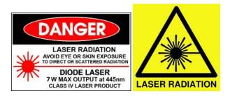
Laser light can cause damage to eyesight and skin if proper laser safety is not used. Always wear the appropriate laser goggles to prevent any laser light, either directly or indirectly to contact the eye. Never expose skin directly to laser radiation. Focused light will increase the safety hazard.
