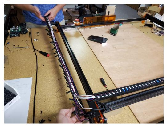
Lay the wires on the Y Axis into the cable chain and close the slots.
