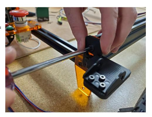
Y axis middle piece. Use the M3 10mm screws. Check the orientation. This is done in the Machine Frame Assembly Step.
