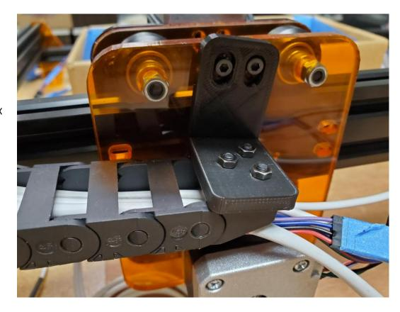
Attach the chain to the back of the X plate.
