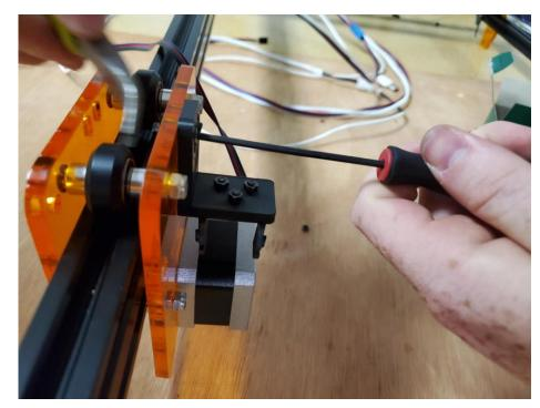
On the 40 x 40 machine, you will need to "tilt" the cable chain mount so the chain does not droop and hit the table. Here is an example of how much tilt you need.
