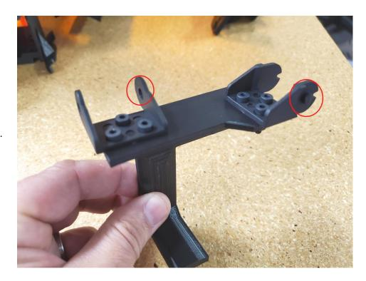
Install the middle Y Axis Cable plastic piece with the two M5 screws and nuts through the right angle pieces.
