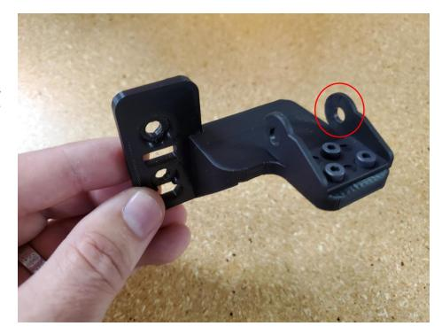
Attach the back Y axis plate with the self tapping screws.
