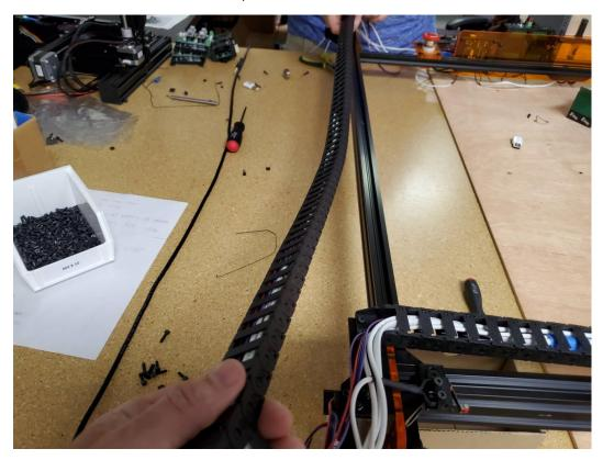
Push the wires under the Y plate and connect the chain to the bracket.
