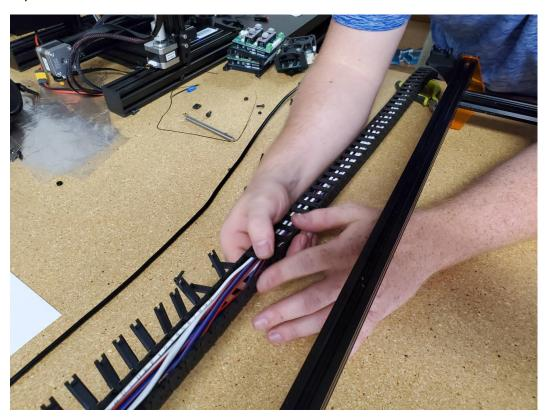
Orient the chain to attach it to the plates.
