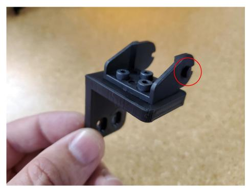
Attach the X Axis piece to the back X axis plate in the top M3 holes. Use the M3 12mm screws and nuts.
