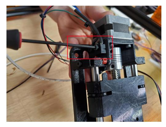
The new Z stage has four M5 15mm screws. They will attach to the X axis front plate.
