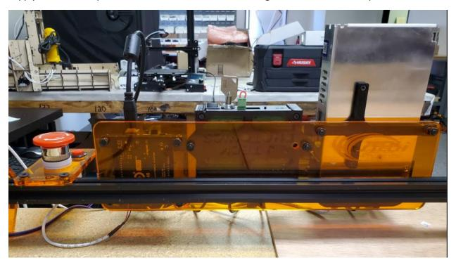
Note the Driver location has changed and the power supply has a new cover on it.
