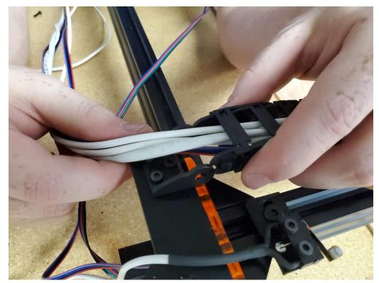
Open the Y axis cable chain slots.
