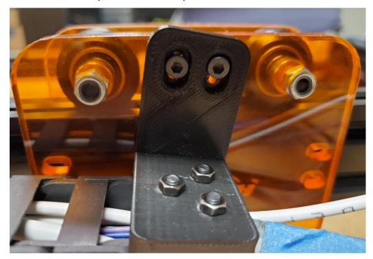
Y Axis Back piece. Use the M3 10mm screws. Make sure the cable chain end piece has a hole in it (female). This is done in the End Plate Step.
