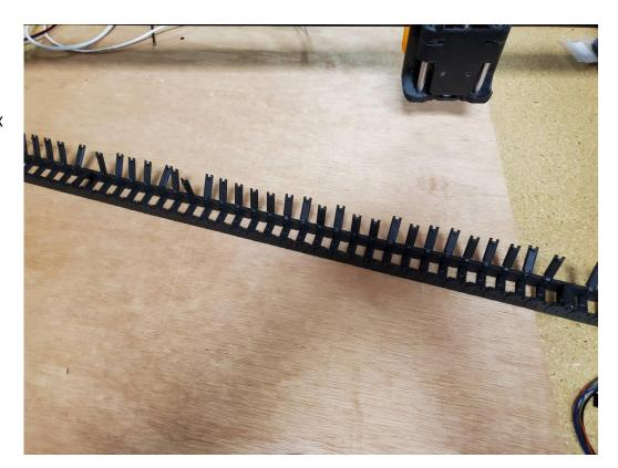
Put the wires from the Z carriage into the cable chain. Make sure the extension cables for the laser and fan are sticking out the end.
