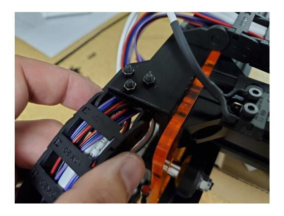
Make sure the cable chain goes through above the motor.
