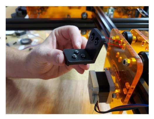
Tighten the M3 screws and nuts on the X Axis plate.
