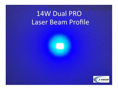
Spot size on wood typical is about 0.006" or less. On Acrylic, it is 0.0045". On tile it is 0.0035".
