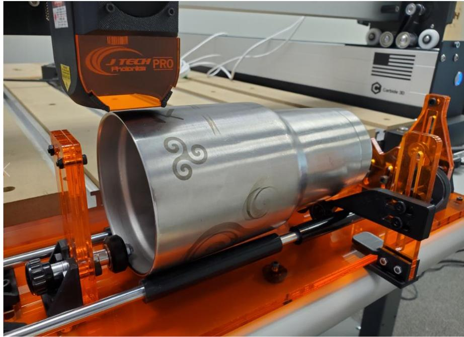
Adjust the back of the cup with the tapered cup holder to allow the side of the cup to be level.
