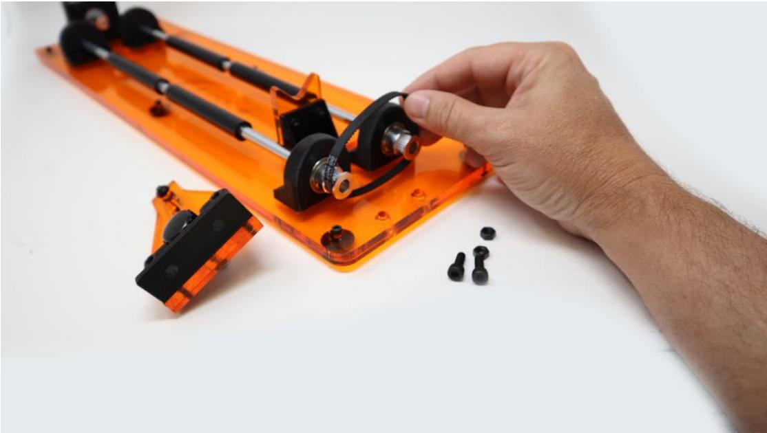
2. Put the screws and nuts to hold the belt tensioner in place.
