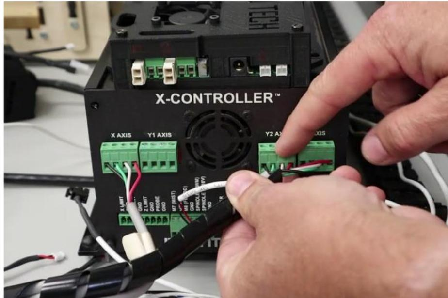
Remove the Y1 connector and replace it with the rotary connector.
