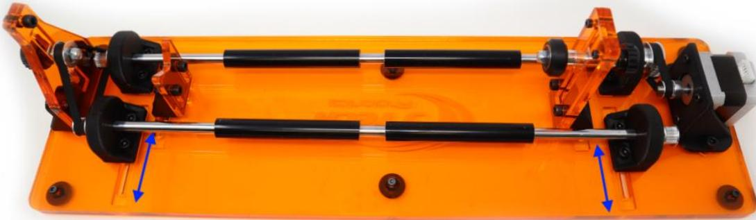
Loosen the screws on both sides to be able to move the rod.
