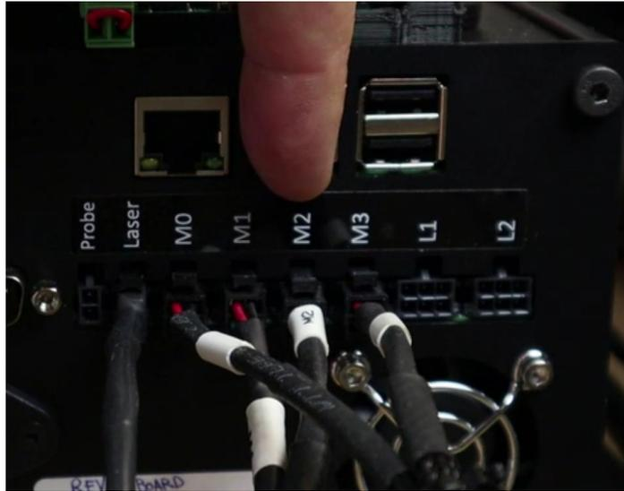
Plug the motor end of the rotary cable into the rotary.
