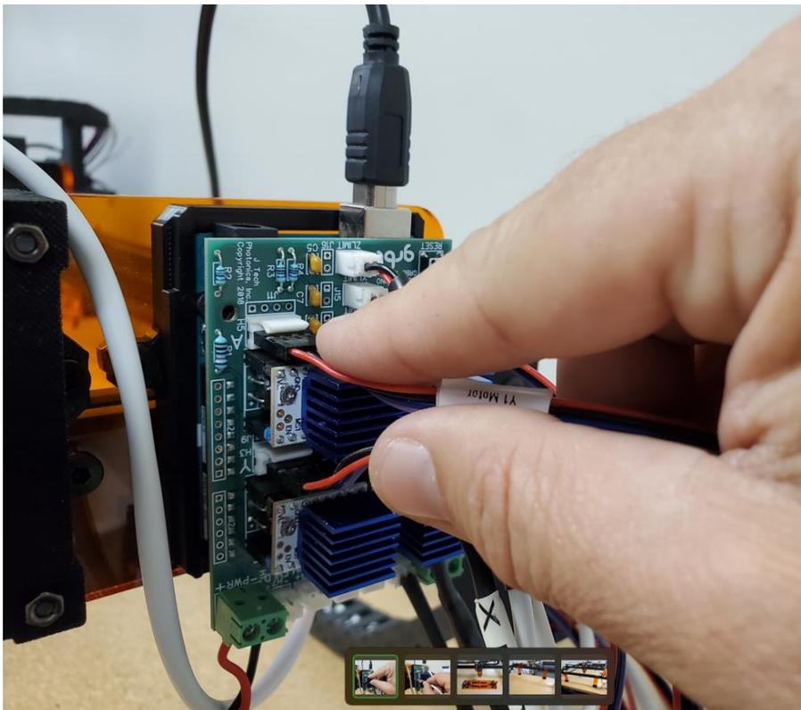
5. Put the rotary cable in the Y position.
