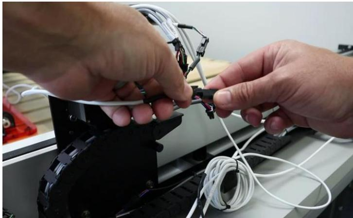
Unplug the Y Right cable and plug in the rotary to it. You can look at the motor on the right side and trace the wires to the Y right connector.
