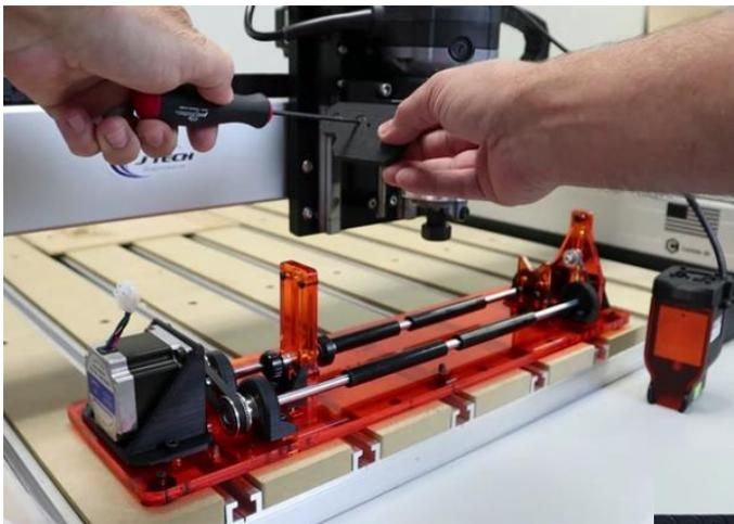
If you don't have the front mount, you can install the side mount for the laser. There are two screws to mount it on the router holder on the left side.
