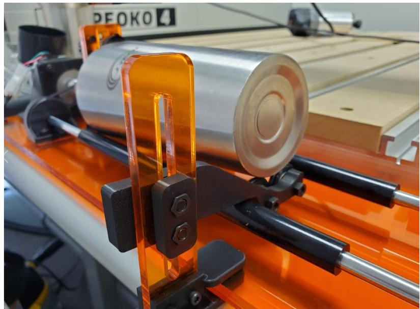
Lay the back of the cup on the holder and adjust the height so the top of the cup is level.
