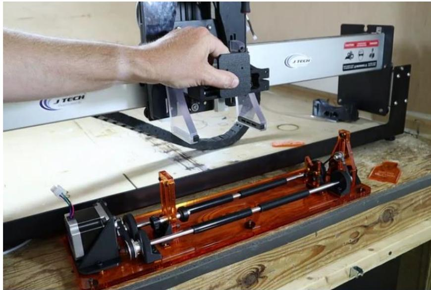
Connect the motor cable for the rotary into the rotary motor.
