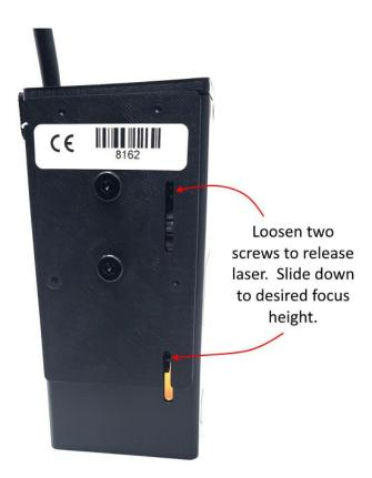
\*There is no need to adjust the factory focus setting of the laser unless you want to do 3D engravings. It is best to leave it at the factory setting.
