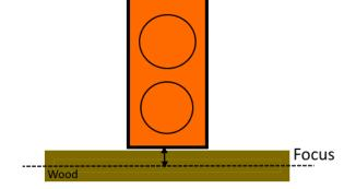
When cutting, set the laser focus to just above the wood to allow the focus to be in the middle or on the bottom of the wood.
