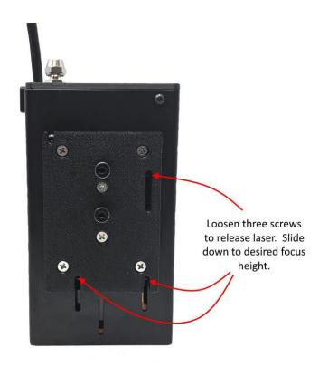
\*There is no need to adjust the factory focus setting of the laser unless you want to do 3D engravings. It is best to leave it at the factory setting.
