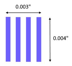
Kerf width (or "line interval" in Lightburn) will be the minimum spot size plus the heat affected zone. This is shown in the following diagram.
