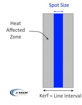
Heat Affected Zone (HAZ) will be different depending on the material and will determine your optimal line interval. Choose your line interval based on how large your kerf is. Some materials like direct metal engraving will have minimal HAZ, so your line interval will be equal to your spot size.
