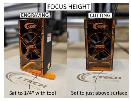
For cutting, we recommend putting the focus at the middle or the bottom of the material. For example, if you are cutting 1/8" material, then set the focus of the laser at 1/8". If you are cutting ½" material or more, then put the laser almost touching the material to allow for the focus to be at the bottom.
