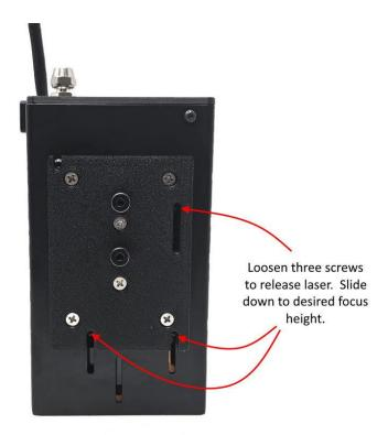
\*There is no need to adjust the factory focus setting of the laser unless you want to do 3D engravings. It is best to leave it at the factory setting.
