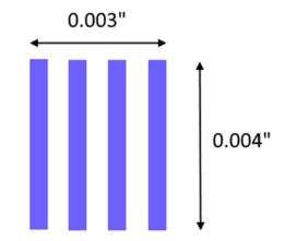
Kerf width (or "line interval" in Lightburn) will be the minimum spot size plus the heat affected zone. This is shown in the following diagram.
