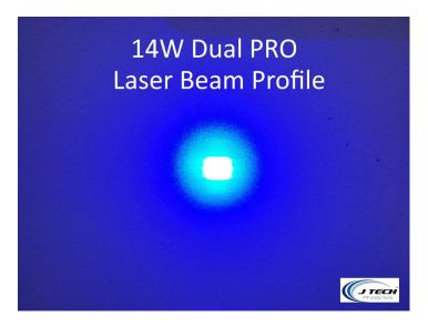
Spot size on wood typical is about 0.006" or less. On Acrylic, it is 0.0045". On tile it is 0.0035".
