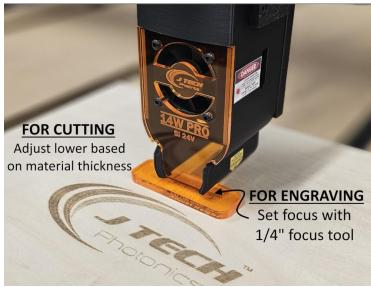
For cutting, we recommend putting the focus at the middle or the bottom of the material. For example, if you are cutting 1/8" material, then set the focus of the laser at 1/8". If you are cutting 1/8" material or more, then put the laser almost touching the material to allow for the focus to be at the bottom.
