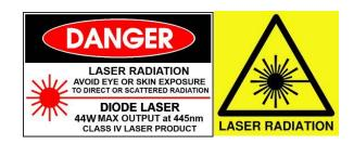
Laser light can cause damage to eyesight and skin if proper laser safety is not used. Always wear the appropriate laser goggles to prevent any laser light, either directly or indirectly to contact the eye. Never expose skin directly to laser radiation. Focused light will increase the safety hazard.
