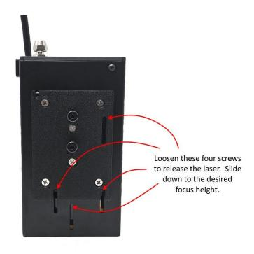
\*There is no need to adjust the factory focus setting of the laser unless you want to do 3D engravings. It is best to leave it at the factory setting.
