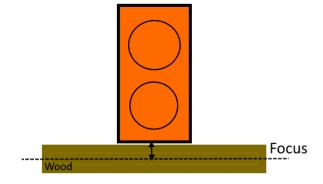
When cutting, set the laser focus to just above the wood to allow the focus to be in the middle or on the bottom of the wood.
