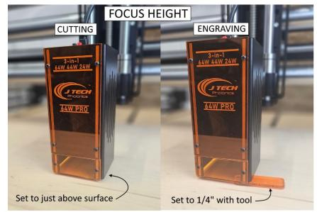
For cutting, we recommend putting the focus at the middle or the bottom of the material. For example, if you are cutting 1/8" material, then set the focus of the laser at 1/8". If you are cutting ¼" material or more, then put the laser almost touching the material to allow for the focus to be at the bottom.
